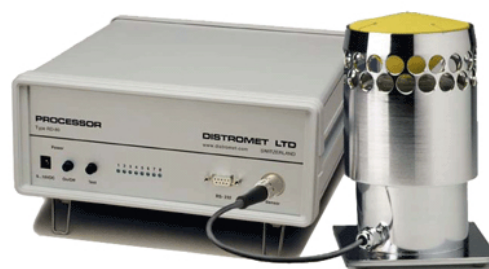
Fig. 5: Impact disdrometer, ©Distromet.
