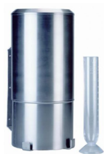
Fig. 3: Accumulation rain gauge type Hellmann, ©BLET-climat, 2017.
