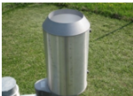
Fig. 4: Tipping bucket rain gauge used by MeteoSwiss, ©MeteoSwiss, 2014c.
