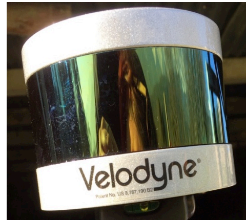
Fig. 10: Lidar VLP-16 used for measurements.
