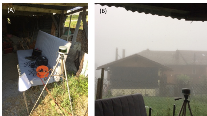
Fig. 11: Set-up of lidar, view from in front (A) and view from inside the shelter (B), ©D.Perrin.
