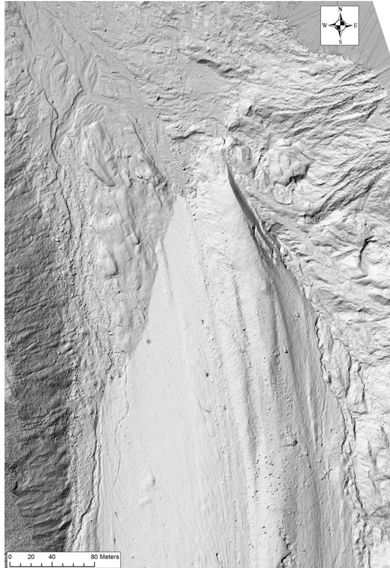
Figure 3.1: High resolution hillshaded digital elevation model obtained using drone photogrammetry, revealing extremely detailed features both on the Haut Glacier d’Arolla and in the proglacial area.
