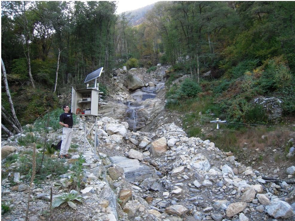
Fig. 5 : Main part of the automated debris-flow monitoring station (2008 - 2009) at the lower 60 m long deflection dam. Two geophones at the upper and lower end of the dam provide information on local front velocities, a radar sensor measures the local flow depth and a video camera in uphill direction captures images of the flow. Data are stored locally and daily transferred by GSM to WSL.
